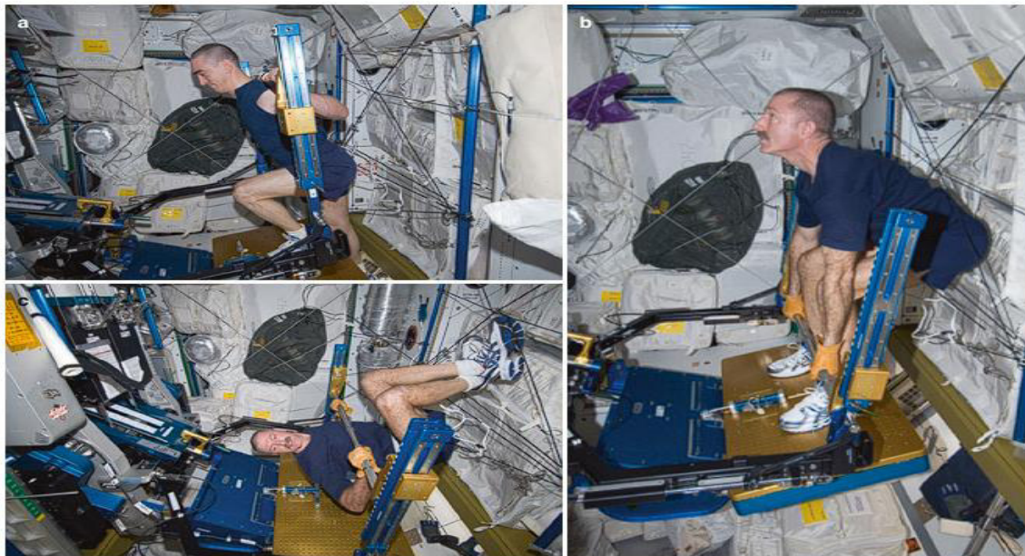
Fig. 20.20 (a–c) Astronauts performing one-legged squats (a), deadlifts (b), and bench press (c) exercises on ISS using the advanced resistive exercise device. (Courtesy of NASA).
