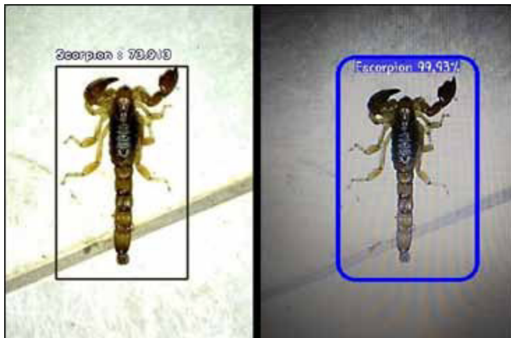
Figure 5. Scorpion detections with YOLOv4 (left) and with MobileNetV2 (right) models
